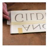
Align the mask to the glass and rub it down taking care to smooth out any air bubbles.
